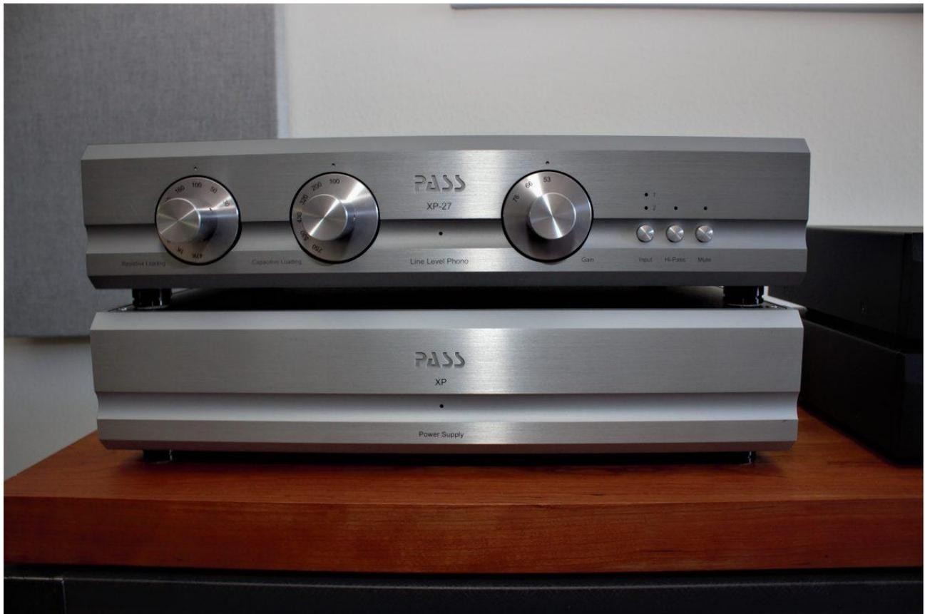
The XP-27 phono preamplifier, like the XP-22, was designed primarily to reduce distortion and noise in the signal path. "Switching and loading is done at higher signal levels," the Pass website proclaims, which improves dynamics, minimizes noise and improves low-level performance. (Both the XP-22 and XP-27 excelled at providing plenty of music information at relatively low volumes.)
